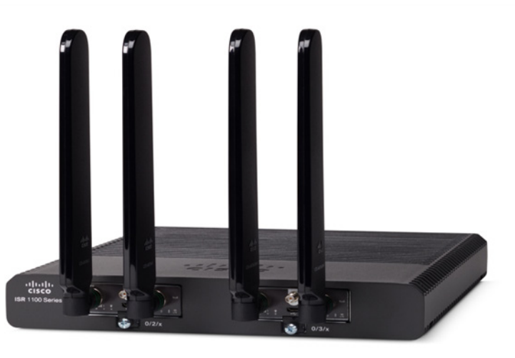
Figure 16. C1109-4PLTE2P front panel with two PIM slots
